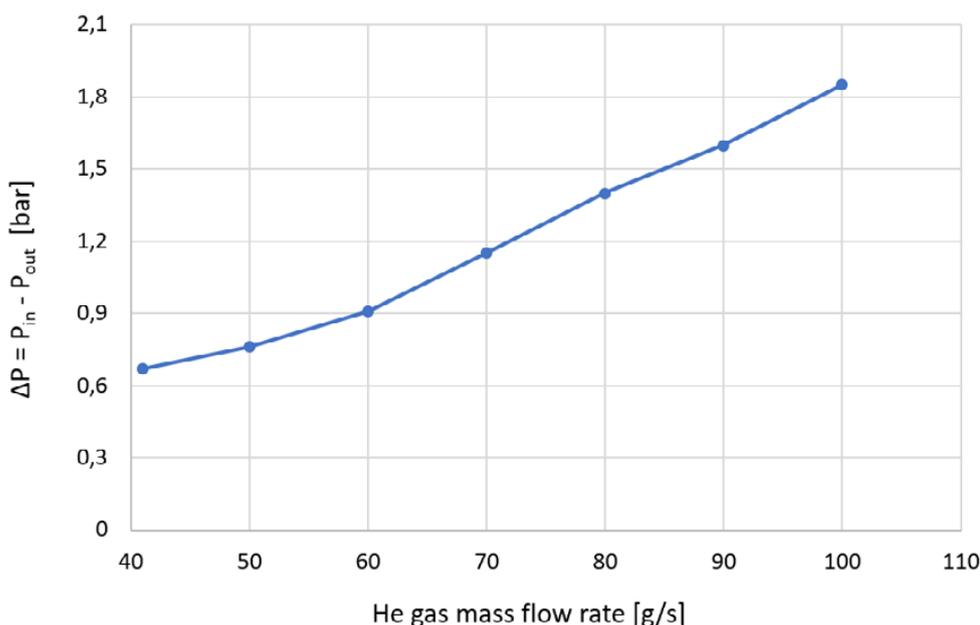
Figure 5 Pressure drop test on PF6 after cool-down at 80 K.
